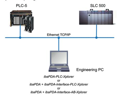
Physically, the connection is established between the *ibaPDA* computer and the PLC-5 or SLC 500 controller via the standard network interface of the computer or an additional network interface card.
