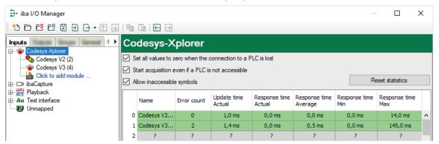
The connected target systems (controllers) are identified by their name or IP address in the first (left) column.
